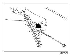
Pull up the release clip, located at the connecting point of the blade and the arm. Then, pull the blade assembly down toward the glass to remove it from the wiper arm.
